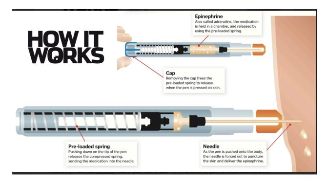
The subject helical compression spring, as designed, is made of A313 stainless steel. The outside coil diameter of the spring is measured as 12 mm. The wire diameter is 0.6 mm.
